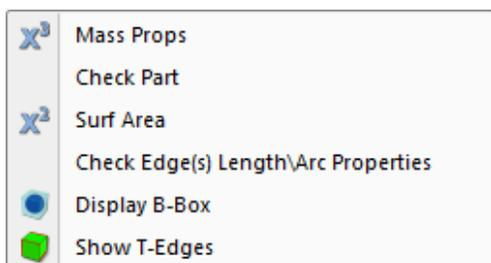
**Check Part** - After selecting a part using the Single Select function, select the Check Part function to perform a geometric integrity check on the selected part. Refer to the output window for repair results.
