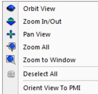
Orbit View - Select Orbit View then depress the left mouse button and slide across the screen to rotate the view.
