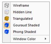
Triangulated - When rendering a scene what is actually being shaded is an approximation of the actual part geometry. These approximations are triangles. Switching to Triangulated mode allows you to see these triangles.
